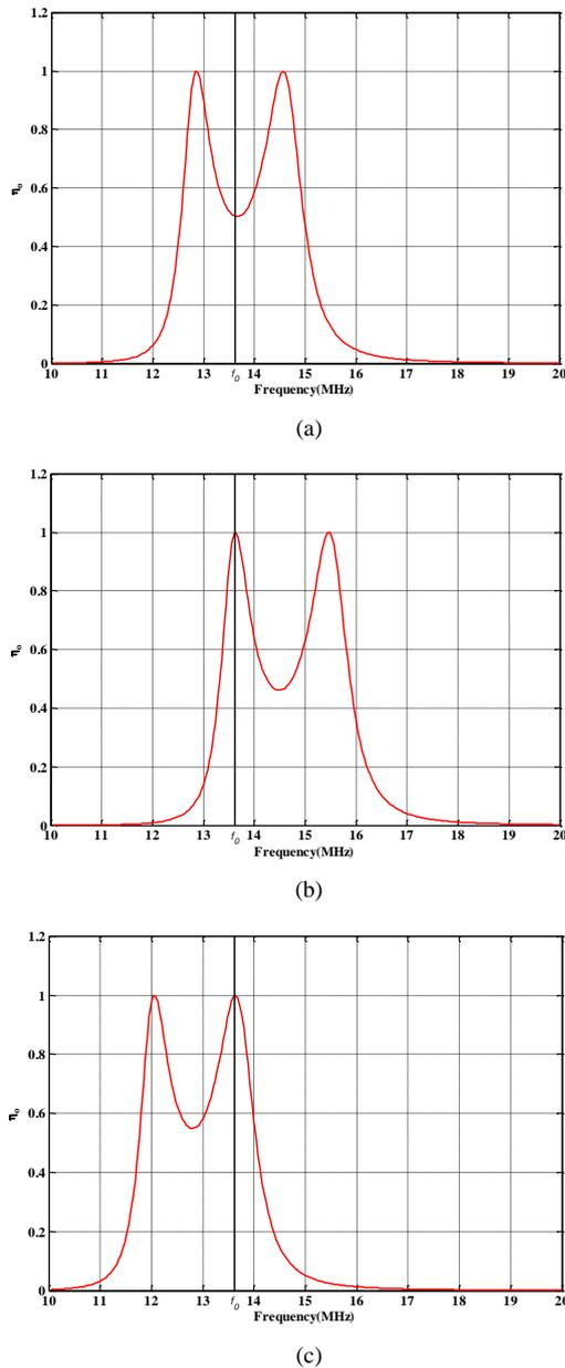
Fig. 9. Power transfer efficiency versus frequency at resonant frequency 13.56 MHz at gap 9 cm: (a) with original values of  $C_1$  &  $C_2 = 13.26$  pF; (b) by tuning  $C_1$  &  $C_2 = 11.78$  pF; (c) by tuning  $C_1$  &  $C_2 = 15.1$  pF.
