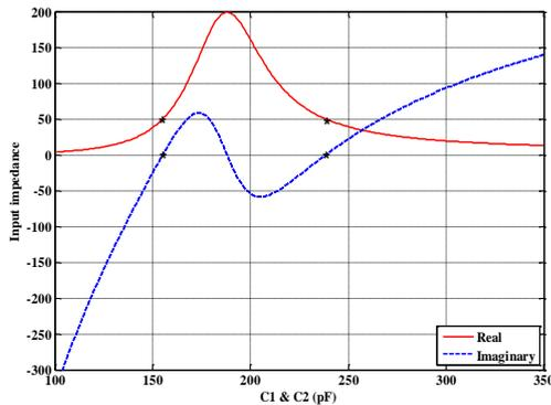
Fig. 7. Input impedance figure by tuning  $C_1$  &  $C_2$  together at gap = 5 cm,  $f_0 = 2.1$  MHz.
