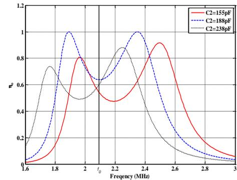
Fig. 5. Power transfer efficiency versus frequency at 5 cm distance tuning  $C_2$  when  $C_1 = 188$  pF.
