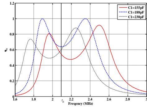
Fig. 4. Power transfer efficiency versus frequency at 5 cm distance tuning  $C_1$  when  $C_2 = 188$  pF.
