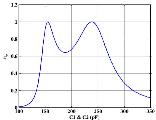
Fig. 6. Power transfer efficiency versus  $C_1$  &  $C_2$  together at gap = 5 cm,  $f_0 = 2.1$  MHz.
