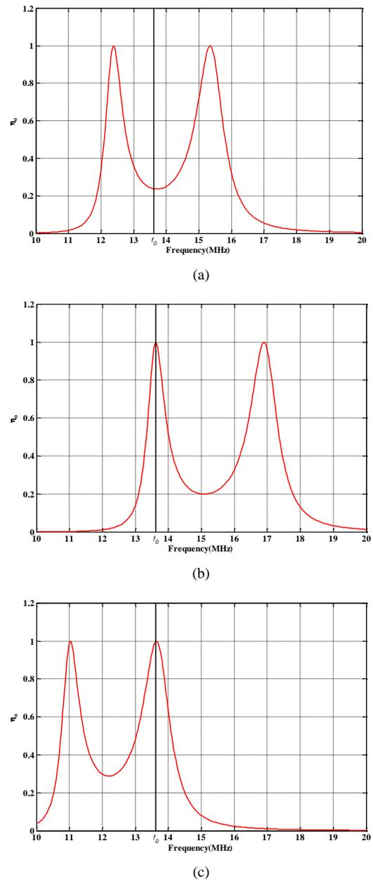
Fig. 10. Power transfer efficiency versus frequency at resonant frequency 13.56 MHz at gap 5 cm: (a) with original values of  $C_1$  &  $C_2 = 13.26$  pF; (b) by tuning  $C_1$  &  $C_2 = 10.95$  pF; (c) by tuning  $C_1$  &  $C_2 = 16.75$  pF.
