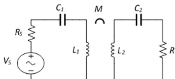
Fig. 1. Equivalent circuit of magnetic coupling wireless power transfer system.
