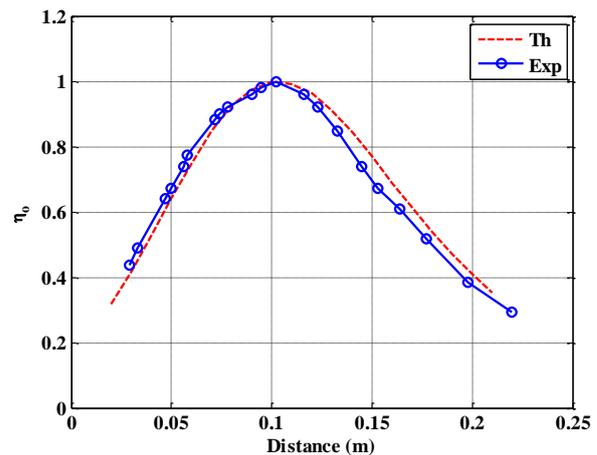
Fig. 2. Power transfer efficiency versus distance at resonance frequency 2.1MHz, RL = 50 $\Omega$ .
