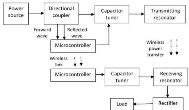
Fig. 11. Block diagram of the suggested symmetric capacitors tuning design.
